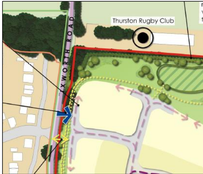
Figure 4: Indicative emergency vehicle access
