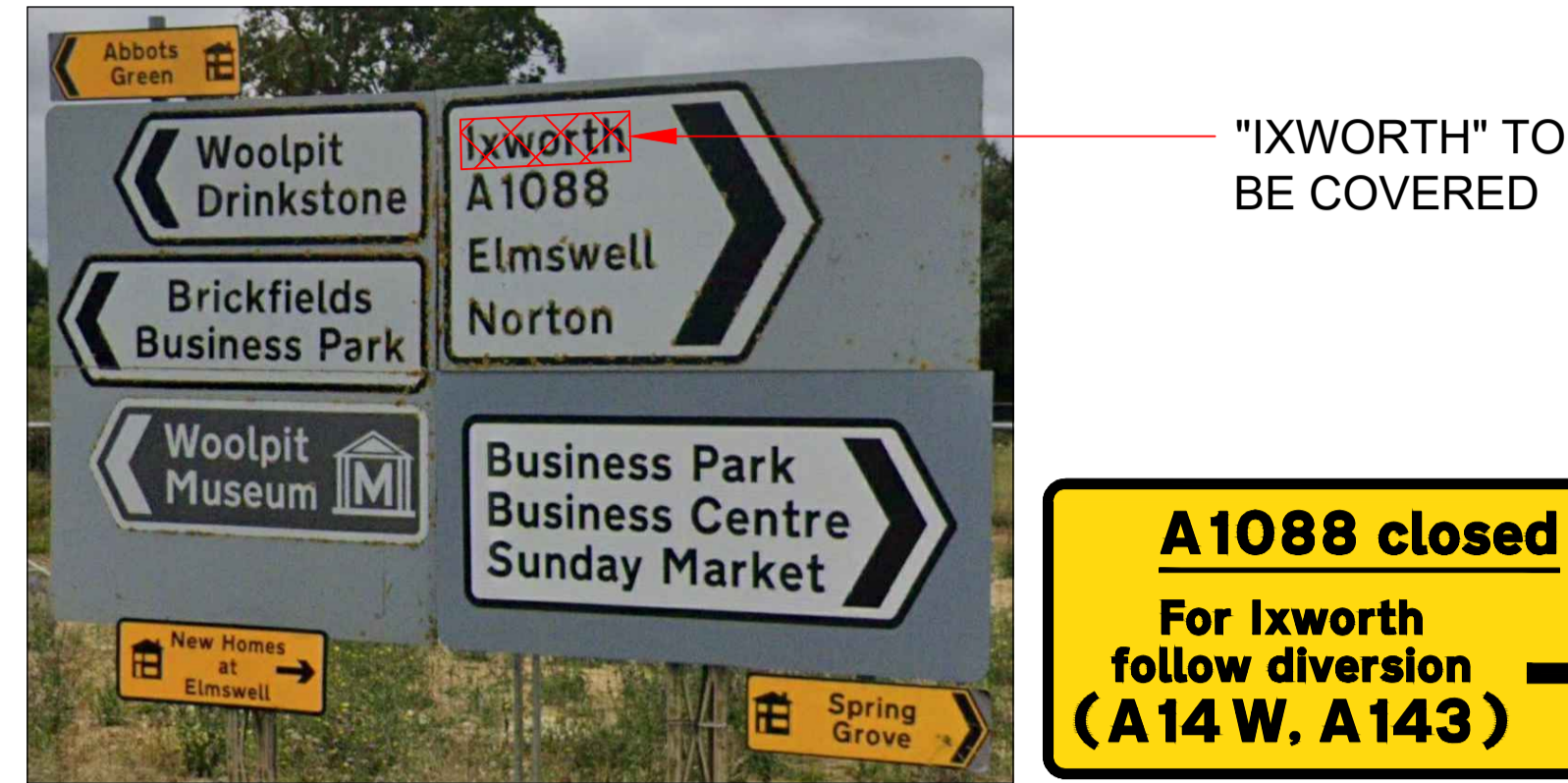
SIGN AT LOCATION 1 WITH ADDITIONAL SIGN REF A8
